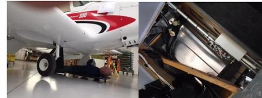
With oleo dampened trailing link using hydraulic foot /hand brakes.
